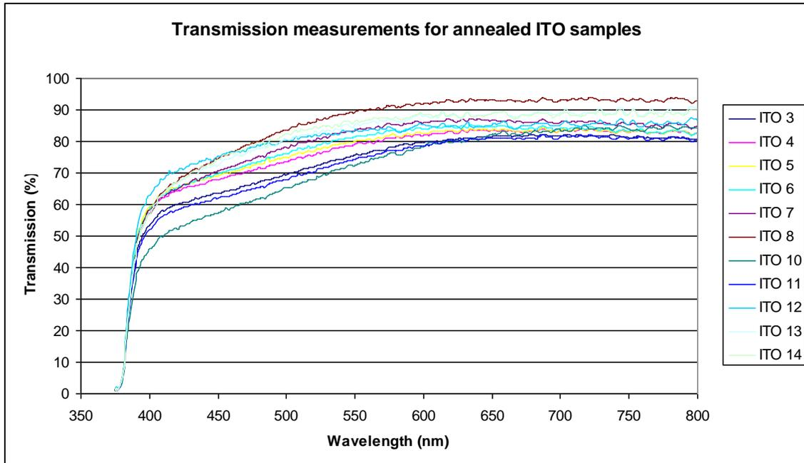
Figure 4. Transmission measurements for ITO film and substrate following after 90 minute anneal at 110° C.
