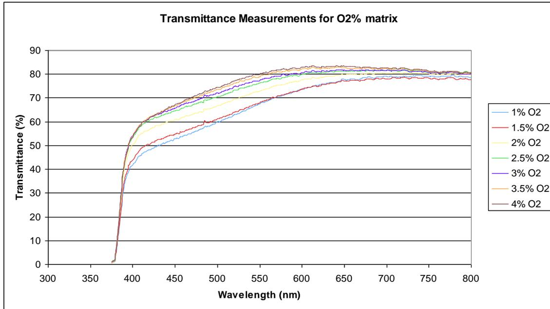
Figure 2. Transmission vs Wavelength for O<sub>2</sub>% matrix. Transmission values are of substrate and ITO film.
