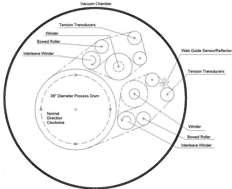
Figure 1. CHA chamber design, web can be run in forward and reverse directions
