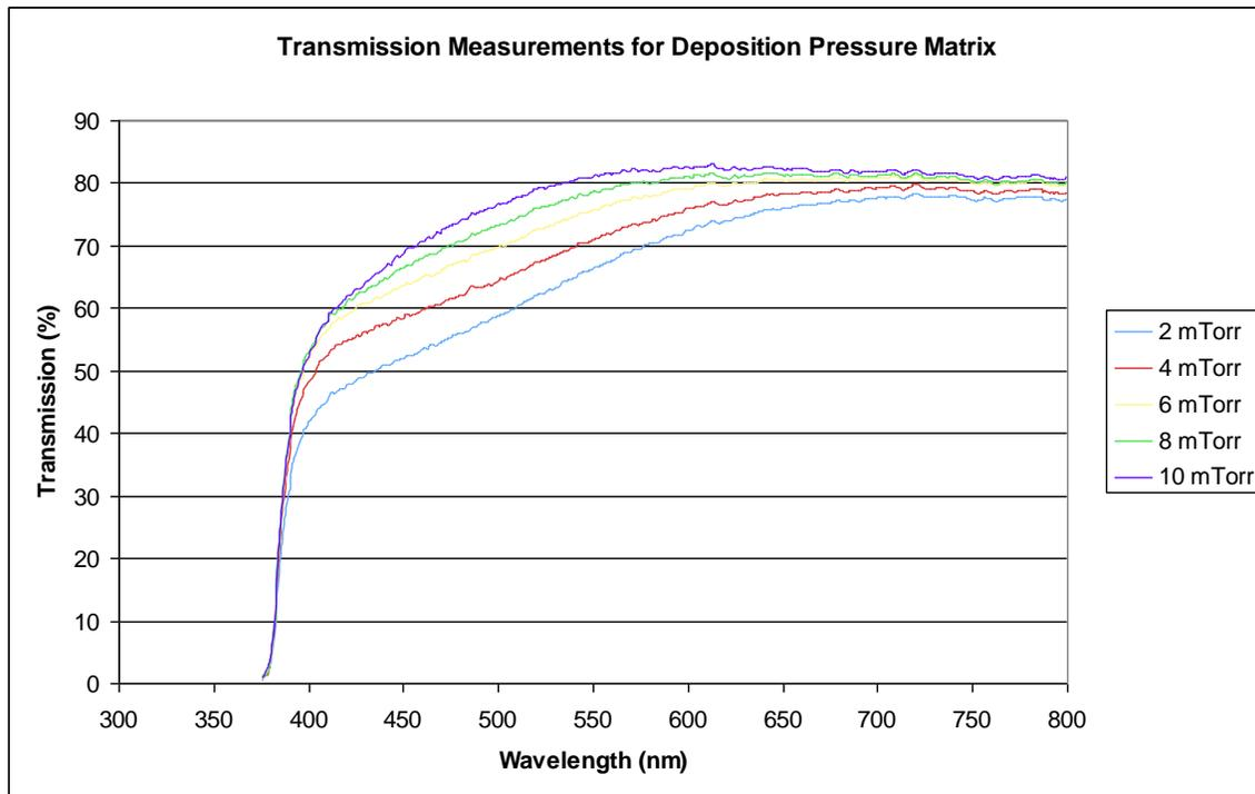
Figure 3. Transmission vs Wavelength for the deposition matrix experiment. While O<sub>2</sub> % has the largest effect on the quality of deposited films it is also known that deposition pressure plays a role in final film quality. We selected 2% O<sub>2</sub> and investigated
