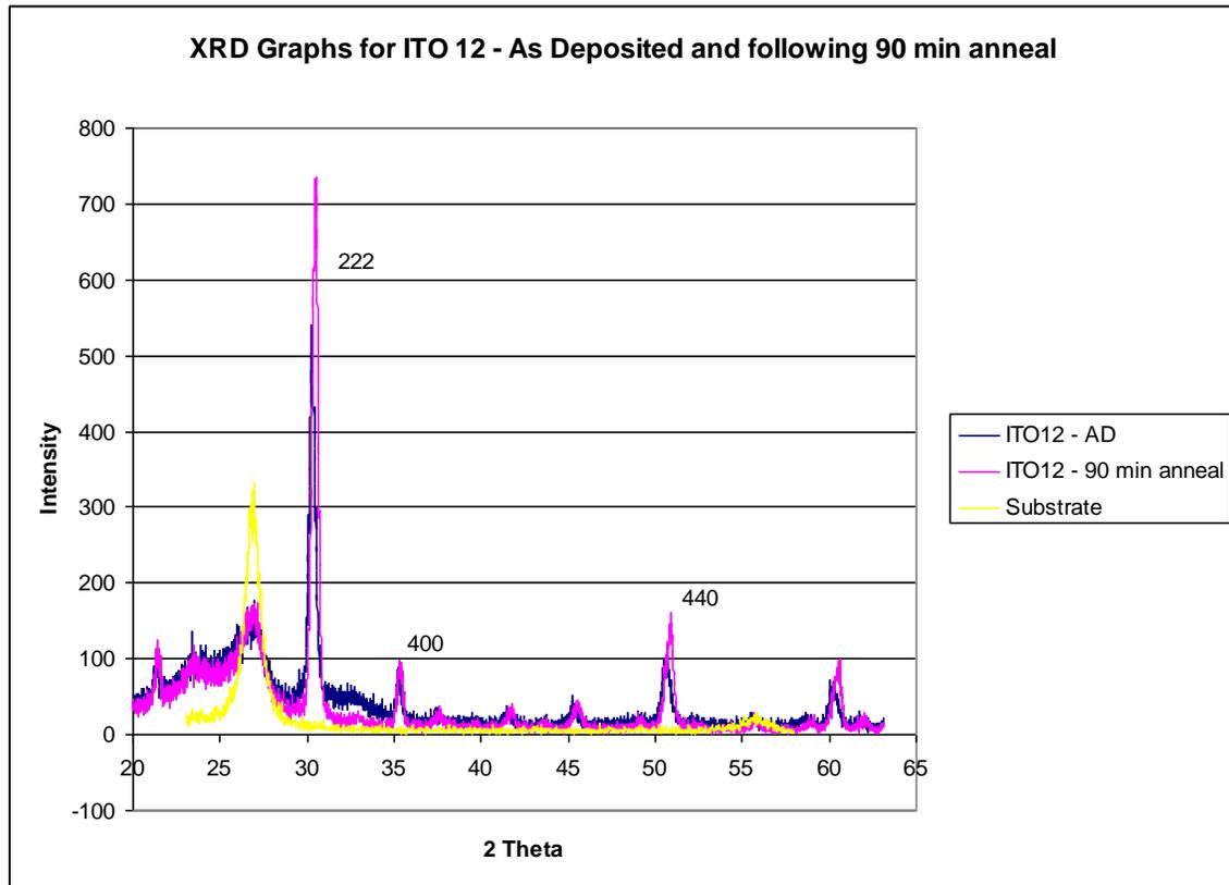
Figure 4. X-ray Diffraction measurement of the PEN substrate, ITO 12 as deposited and ITO 12 after 90 minutes of annealing.
