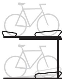
Typically used for high-density indoor parking. Performance varies widely. Models for public use include lift assist for upper-tier parking. Recommend testing before purchasing. Creates safety concerns not inherent to on-ground parking, and requires maintenance for moving parts.
