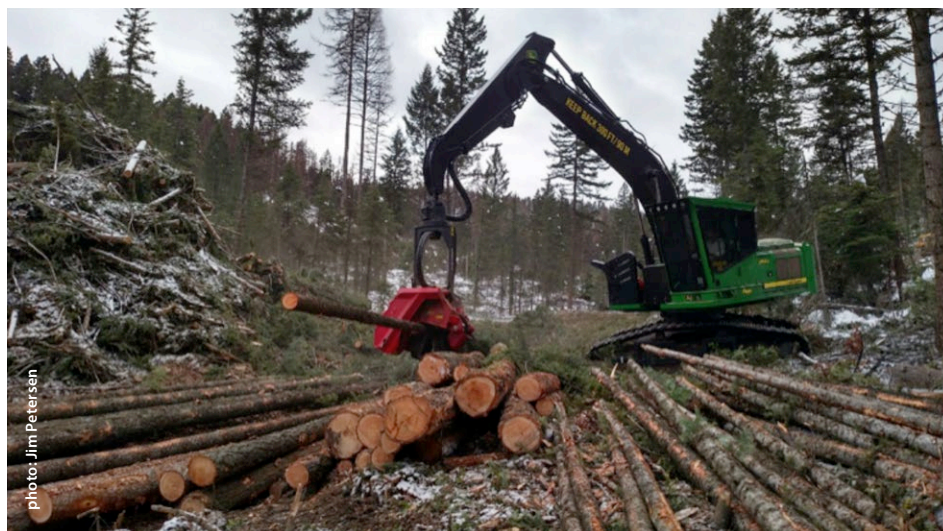
The business end of Swanstrom Logging, processing trees by length and diameter, on private land west of Kalispell, Montana. Machines like this are essential tools in forest thinning and restoration work.
