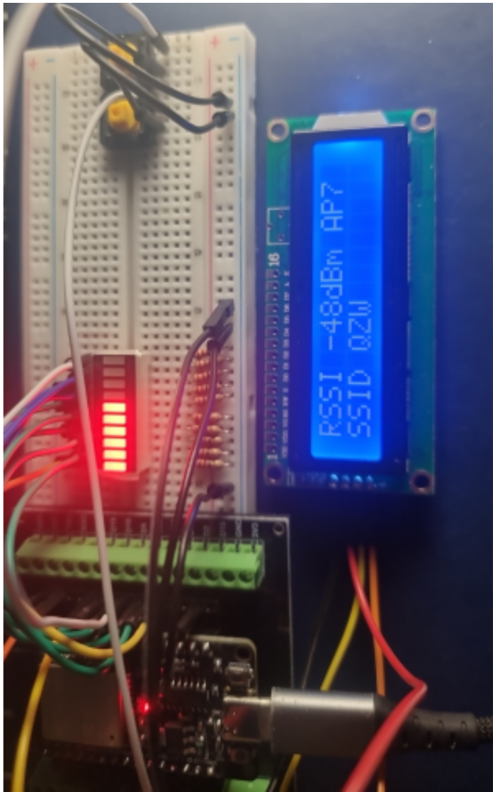
Figure 10: Early rapid prototyping stage using loose jumper wiring with LED bar and LCD output.
