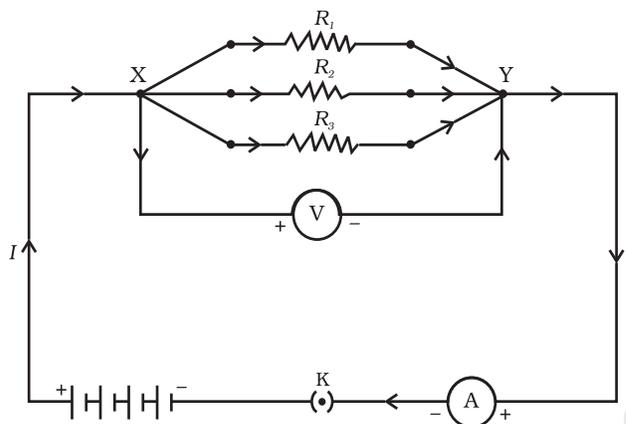
**Figure 11.7** Resistors in parallel
