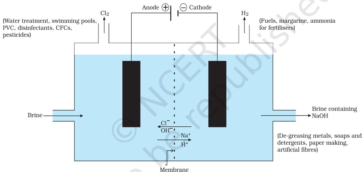
**Figure 2.8** Important products from the chlor-alkali process
