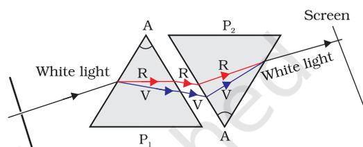
**Figure 10.6** Recombination of the spectrum of white light
