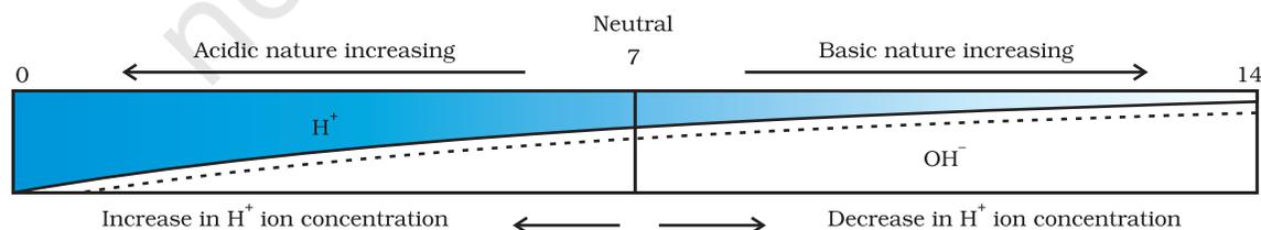
**Figure 2.6** Variation of pH with the change in concentration of H<sup>+</sup>(aq) and OH<sup>-</sup>(aq) ions
