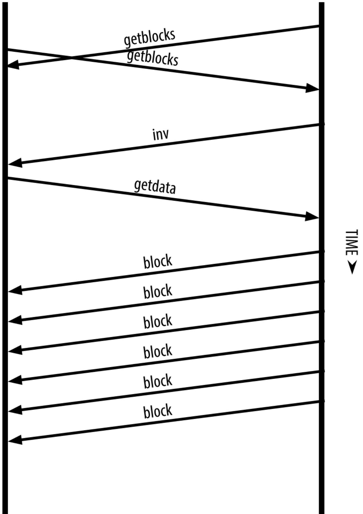
Figure 53. Node synchronizing the blockchain by retrieving blocks from a peer
