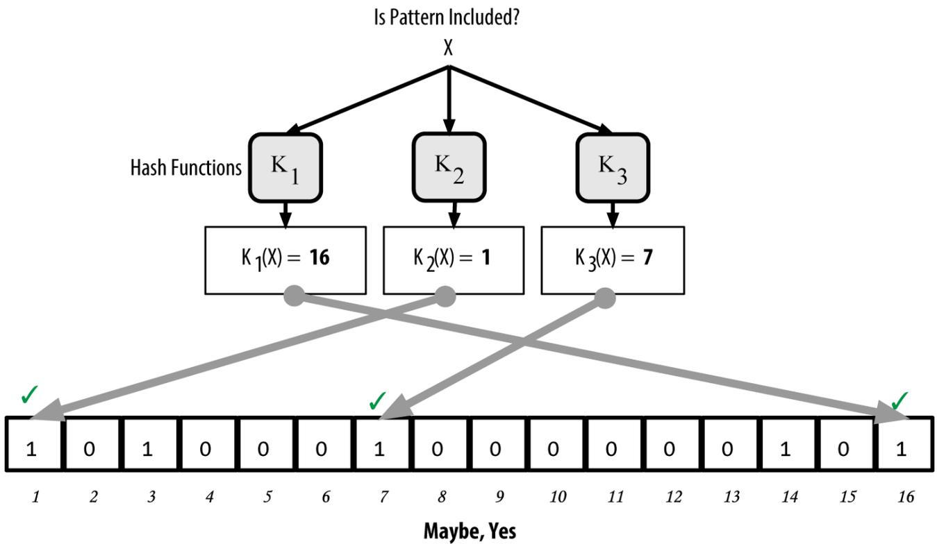
Figure 58. Testing the existence of pattern "X" in the bloom filter. The result is a probabilistic positive match, meaning "Maybe."
