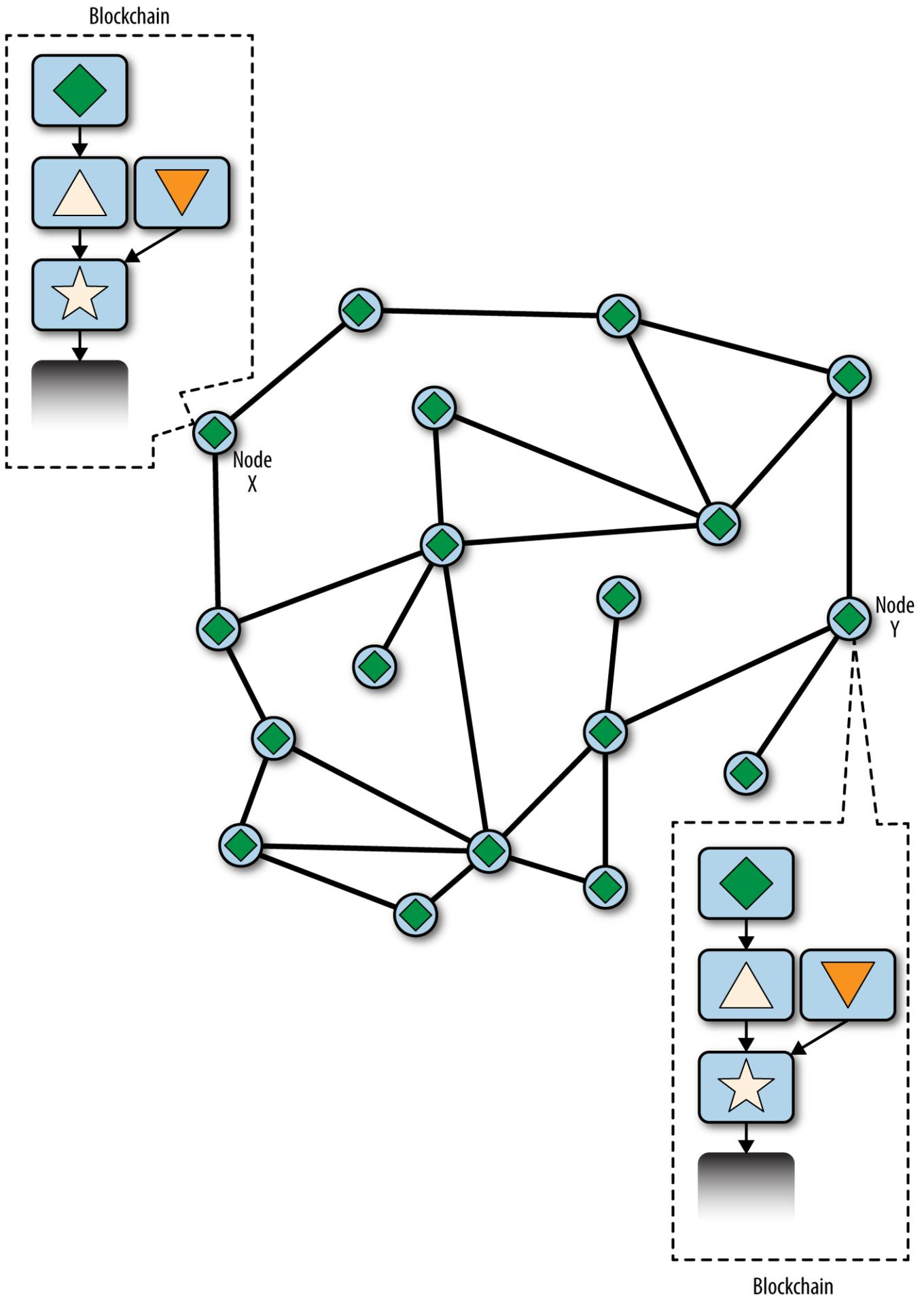
Figure 70. Visualization of a blockchain fork event: the network reconverges on a new longest chain
