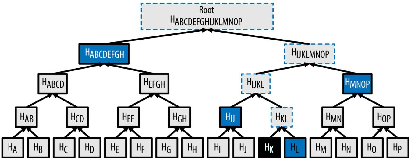
Figure 64. A merkle path used to prove inclusion of a data element
