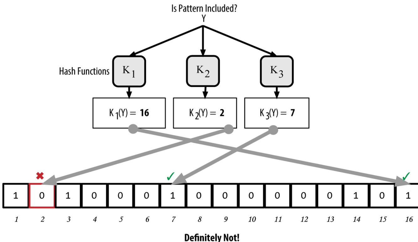
Figure 59. Testing the existence of pattern "Y" in the bloom filter. The result is a definitive negative match, meaning "Definitely Not!"
