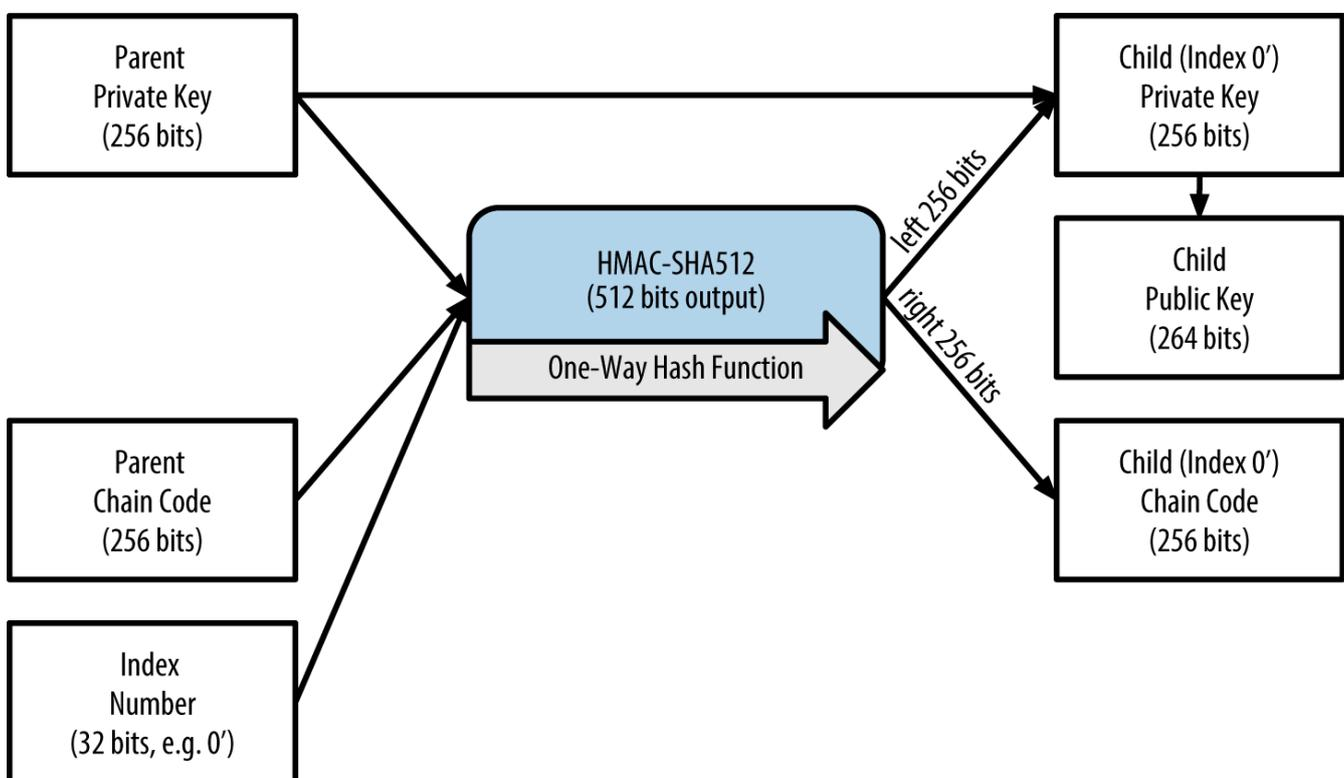
Figure 38. Hardened derivation of a child key; omits the parent public key
