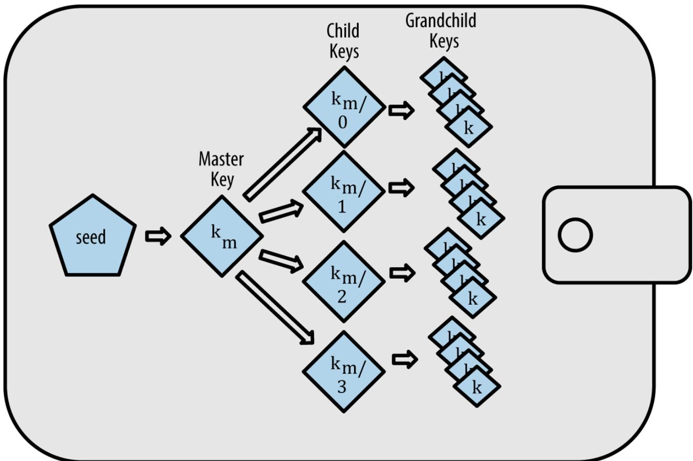
Figure 28. Type-2 HD wallet: a tree of keys generated from a single seed
