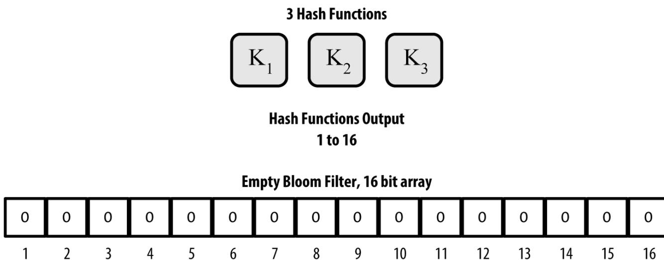
Figure 55. An example of a simplistic bloom filter, with a 16-bit field and three hash functions
