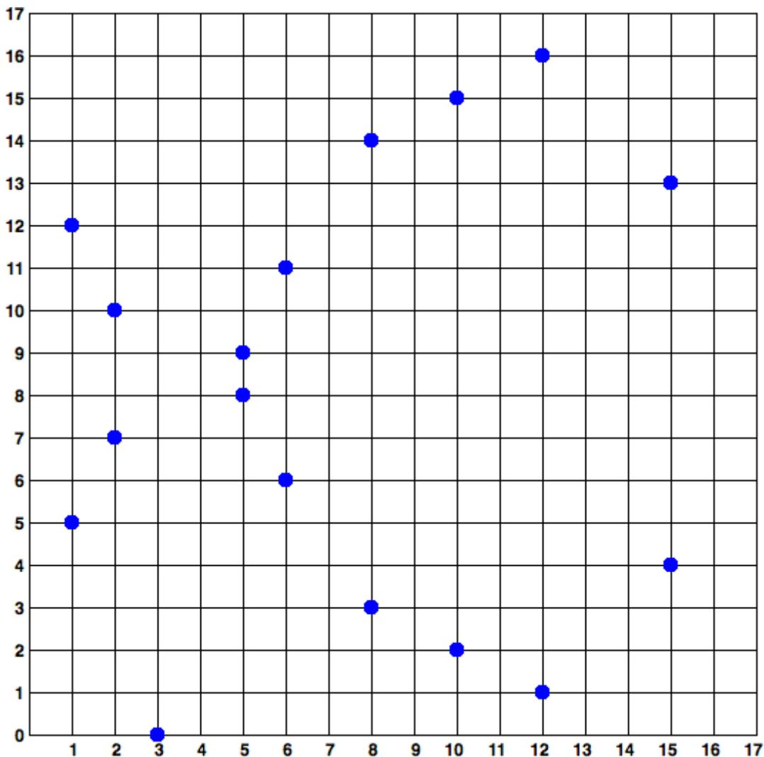
Figure 16. Elliptic curve cryptography: visualizing an elliptic curve over  $F(p)$ , with  $p=17$
