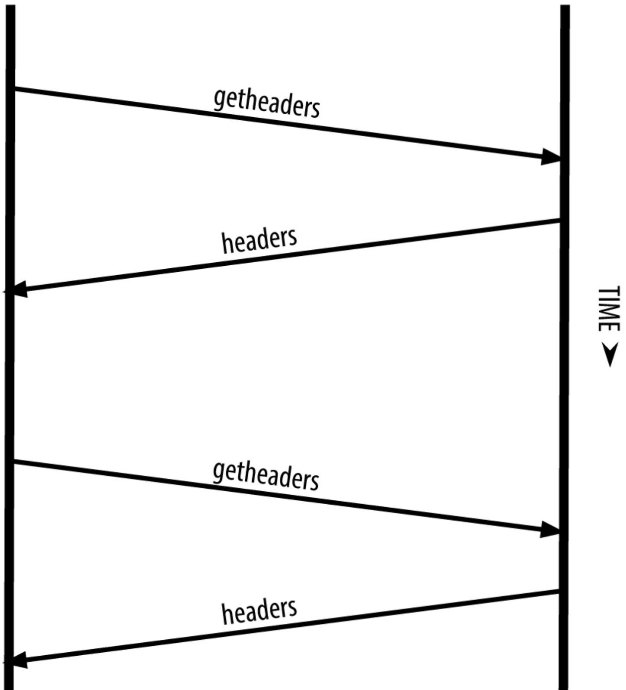
Figure 54. SPV node synchronizing the block headers
