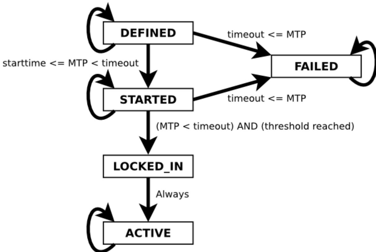
Figure 74. BIP-9 state transition diagram
